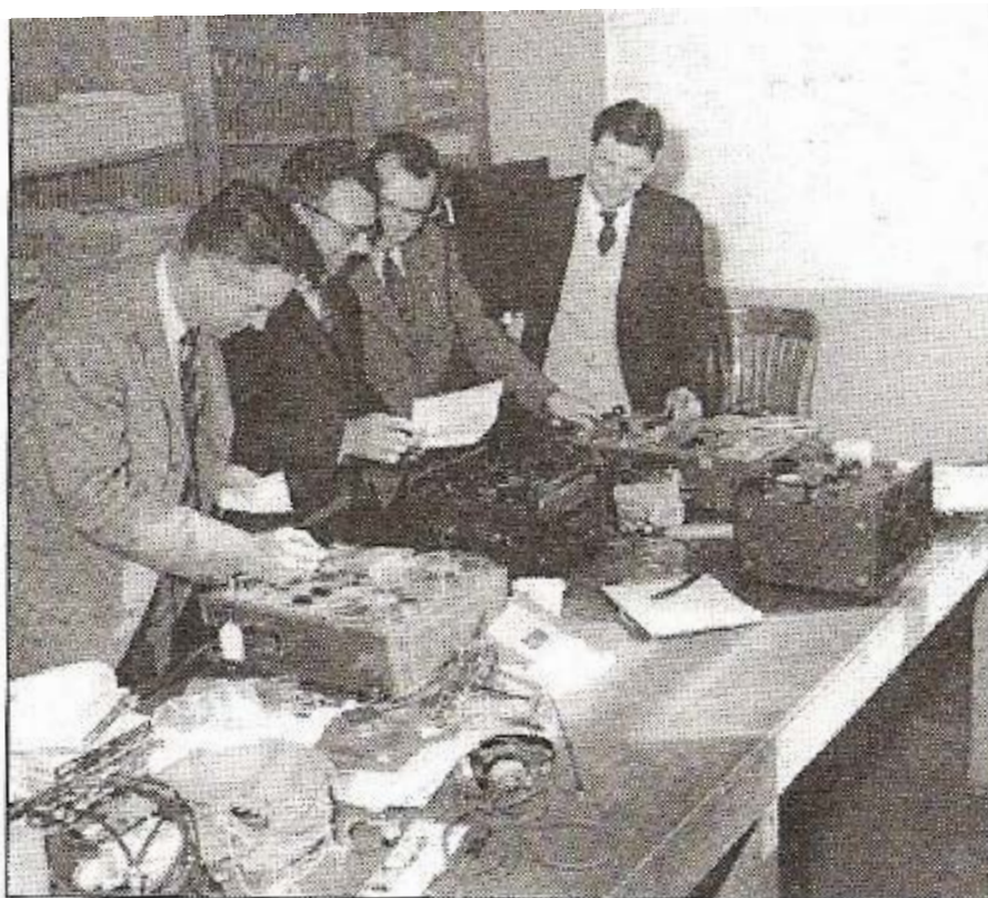
Some of the Noise Measurement Equipment taken to Paris for the Caravelle study. This photo is offered primarily to show the bulky equipment used in those days (1957). The Ampex magnetic tape recorders worked only on 60-Hz AC (we called it 60-cycle in those days), and we had to take two sets of auto storage batteries and converters to produce power while we recorded out in the middle of the corn fields. In the photo, from the left: Laymon Miller, Leo Beranek, and the two Sud Aviation engineers who were our assistants while we were there.
