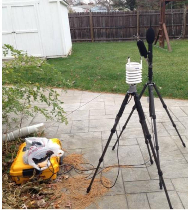
Figure 2: Sound Level meter (unit in yellow case) with external microphone and separate weather station
