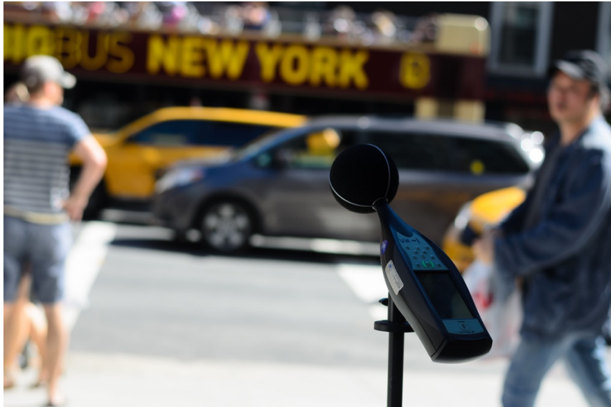
Figure 1: Sound Level Meter placed on tripod measuring noise outdoors
