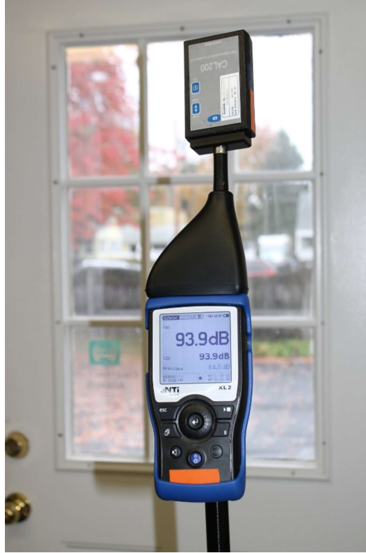
Figure 1: Sound level meter with calibrator seated on microphone.
